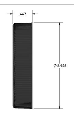
HATCHED AREA & RIBS LITE STIPPLE FINISH UNSPECIFIED AREAS FINISHED SPI-B2 POLISH
